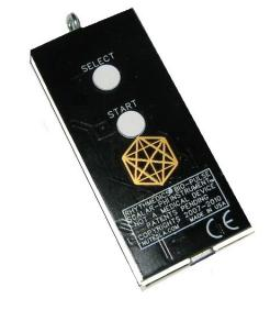
The white dome switches must be pressed until you feel a slight 'give' in the switch, and a soft click may be heard as well. The dome switches are very resilient and it is not possible to press them too hard.
