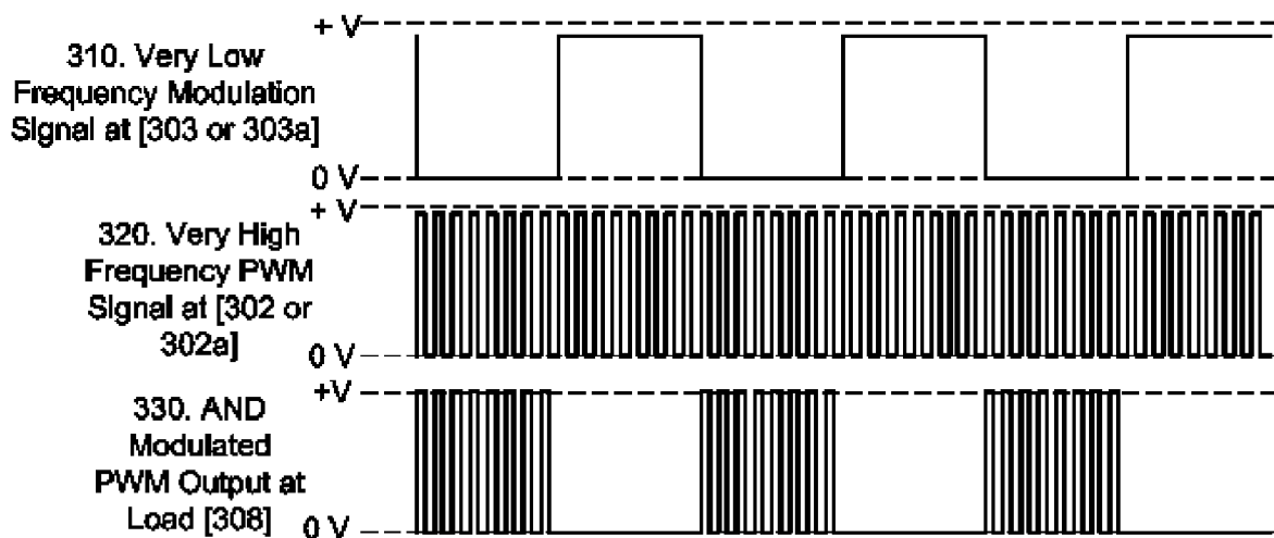
Figure 3b. Prior Art Waveforms– Mono-Polar AND Modulated PWM Pulses
