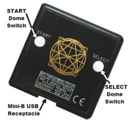
While the dome switches are very sturdy and rated for being pressed hundreds of thousands of times, they can be dislodged if pushed from the side instead of straight down, or even peeled off. To protect the dome switches from rough handling and moisture the back of the Metronome has been sealed with a durable clear tape. The tape can be replaced if it wears through.
