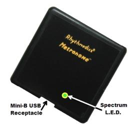
recognizes the charger being connected. Metronome is now in its Standby recharging mode and will flash Green every two and a half minutes to confirm it is charging. If the battery was fully discharged Metronome will begin operating as indicated by flashing its SLED through a series of six colors and then a seventh flash to indicate the running preset. If this
